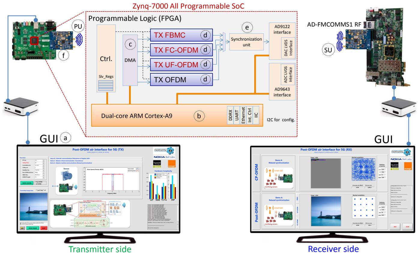
Fig. 1. Demonstration setup with front-end interface.
